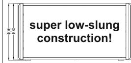
extremely compact and truck space saving design 2 dimension optimized for Euro-pallet norm truck upright loading: 6 x 40cm = 240cm width flat loading: 3 x 80cm = 240cm width 3 rows upright stacked = 240cm width / 240cm height flat and upright loading can be combined 1 x width (80cm) = 2 x height (40cm) 1.125m (incl. caster) loading length up to 18 cabinets 1.125m loading length up to 54,000W /162,000W peak
